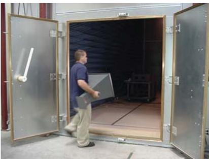
Entry doors are 6' x 7' and can easily be made into 8' x 8'
