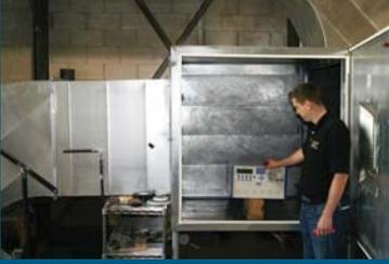
Today's global deployment of electric and electronic equipment used to support military and avionics related activities has resulted in expanded environmental testing requirements for blowing sand and dust compliance. To support these requirements, D.L.S. has upgraded their environmental testing capabilities for MIL-STD-810 G, Method 510 and RTCA DO-160 G, Sec 12 for Sand and Dust Exposure. Large products can be accommodated by D.L.S.'s state of the art equipment.
