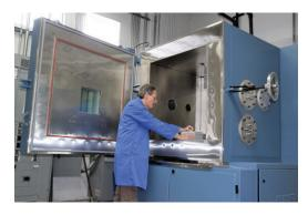
D.L.S. offers compliance testing on Aviation and Avionics platform applications for EMI/EMC, Environmental, Power Quality, and other applicable services. The list of accredited standards includes RTCA/DO-160 for Electromagnetic Compatibility, Lightning, HIRF and Environmental requirements. RTCA/DO-160 defines a series of minimum test conditions (categories) and applicable test procedures for commercial airborne equipment.
